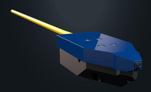
Photon assisted cutting (PAC) by laser is an approach to improve or even enable diamond turning of brittle materials such as infrared optics or tungsten carbide molds. Innolite has developed a new tooling system combining the diamond tool with glass fibre for laser light guidance.
