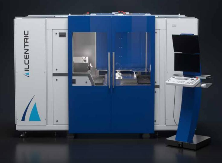
Based on the experience with the ILCENTRIC300, the ILCENTRIC500 has been developed for aligning large lenses with diameters of up to 400 mm. Furthermore, the machine offers space to integrate additional, permanently equipped measuring technology or processes such as the engraving of reference marks, the milling of reference grooves or automated assembly using robots. The ILCENTRIC does not use a conventional center chuck, but a unique dynamic
