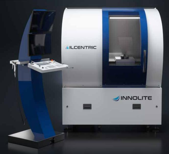
The ILCENTRIC300 is the leading ultra-precision machine platform for high-performance alignment of mounted lenses with diameters of up to 250 mm. Various integrated optical and tactile sensors enable the centering of all relevant modern optics. The ILCENTRIC does not use a conventional center chuck, but a unique dynamic turning process to correct the alignment of the optical axes from lens to frame.
