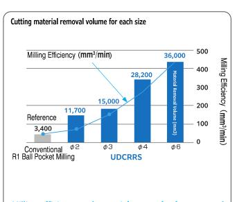
Milling efficiency and material removal volume exceeds the conventional tool.
