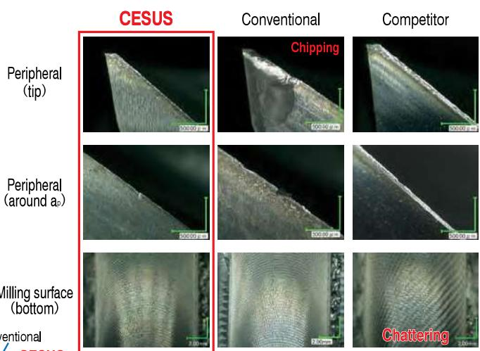
CESUS offers stable milling with less chattering under highly efficient conditions.
