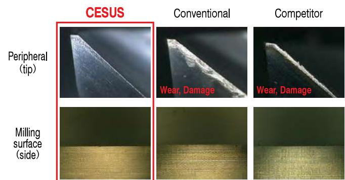
CESUS offers longer tool life with less wear and damage after 120 min of milling! Great surface finish without chattering!
