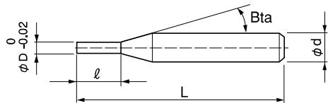
The shank taper angle shown is not an exact value and to avoid contact with the workpiece, we recommend the user controls the precise value of this angle. Shank taper angle should not make contact with the work piece.
