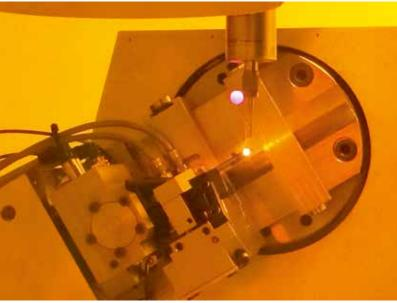
Laser sharpening generating no efforts on the tool, the mass and the kinetic of the machine have been developed specifically to ensure very fast and precise movements.
